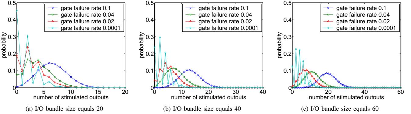
Fig. 3. Output distribution of NAND multiplexing unit with 1 restorative stage under different gate failure rates and I/O bundle sizes
