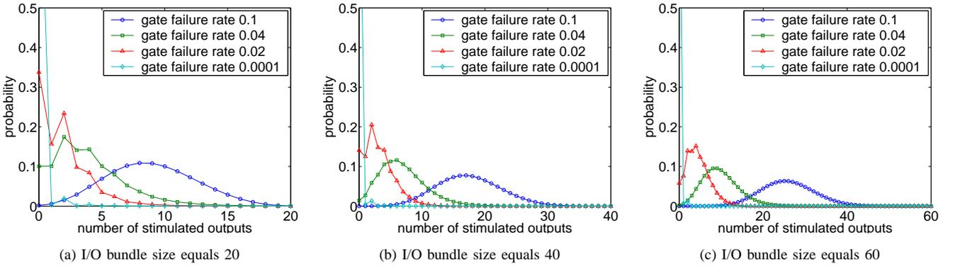
Fig. 4. Output distributions of NAND multiplexing unit with 4 restorative stages under different gate failure rates and I/O bundle sizes
