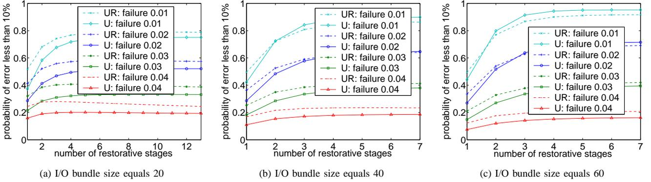
Fig. 6. Probability that at most 10% of the outputs of the overall system are incorrect for different I/O bundle sizes (large probability of failure)
