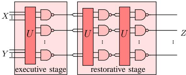
Fig. 1. A NAND multiplexing unit
