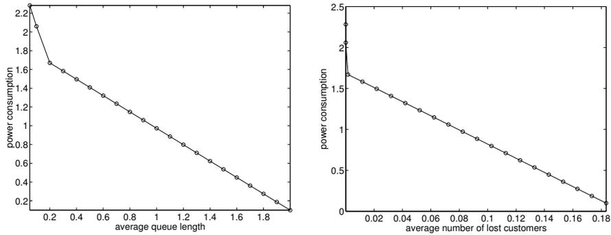
**Fig. 2.** Power versus performance for the disk-drive
